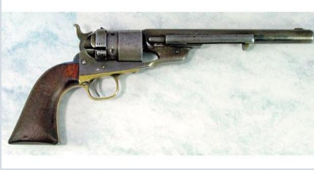
The Colt Peacemaker was not the first Colt that used metallic cartridge to be used by the U.S. Army. In 1872 1200 of the Colt 1860 Richards Conversion revolvers in .44 Colt were purchased to be tested for possible use by the Army. The basis for these .44 conversions was the Model 1860 Army .44. The method used what was called the Richards Conversion, after the Colt engineer who developed it. Colt's Richards
